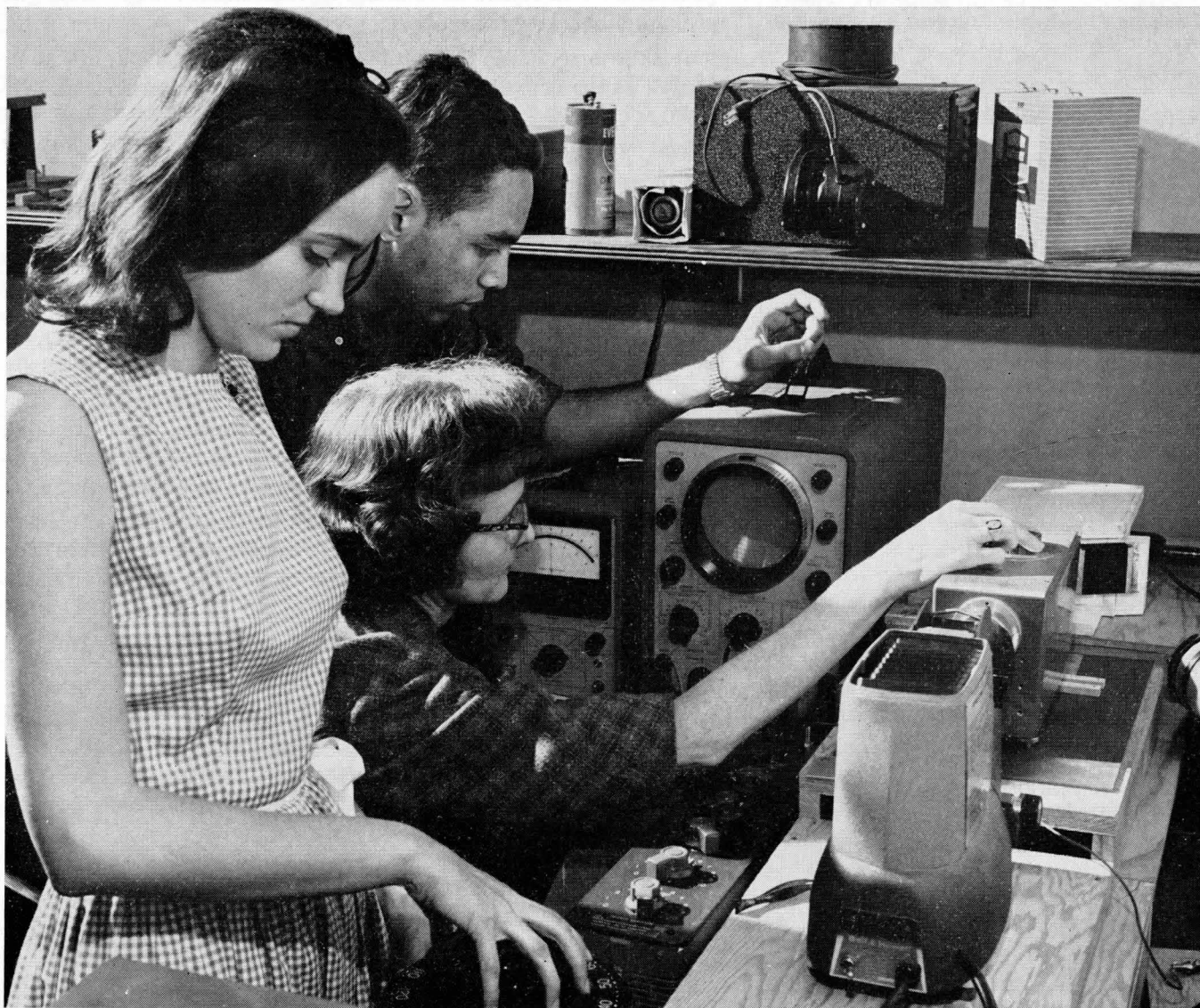
Professor Kennedy with physics students measuring infrared absorption of zinc sulfide phosphor.
