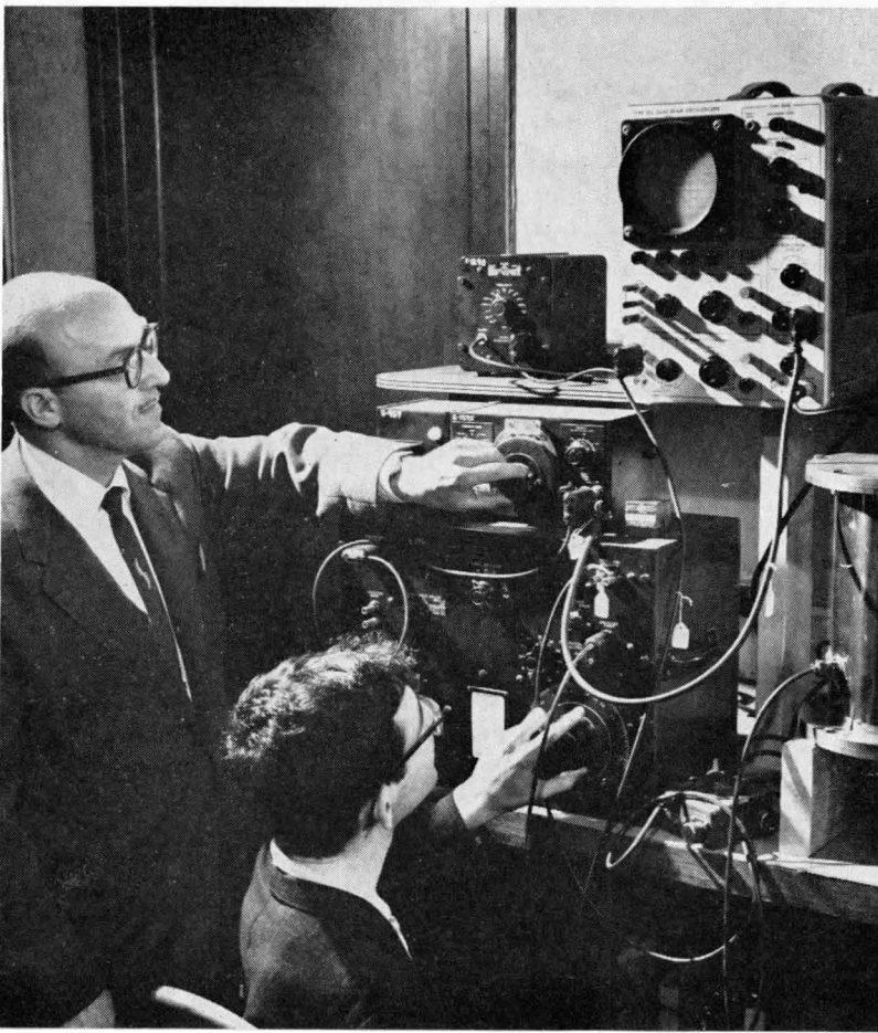
Mr. Balkin, Science Technician, and physics student measuring the light emission of a zinc sulfide phosphor.
